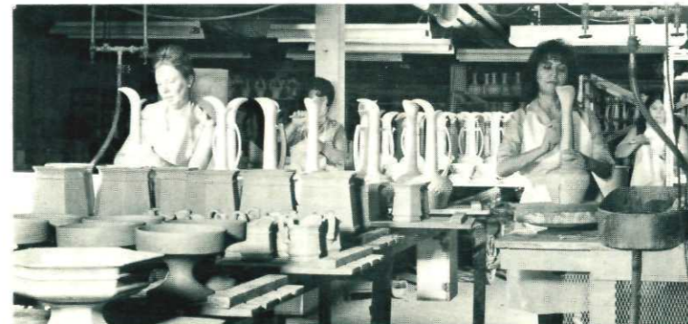
All mold marks and any other slight imperfections are eliminated by hand finishing.
