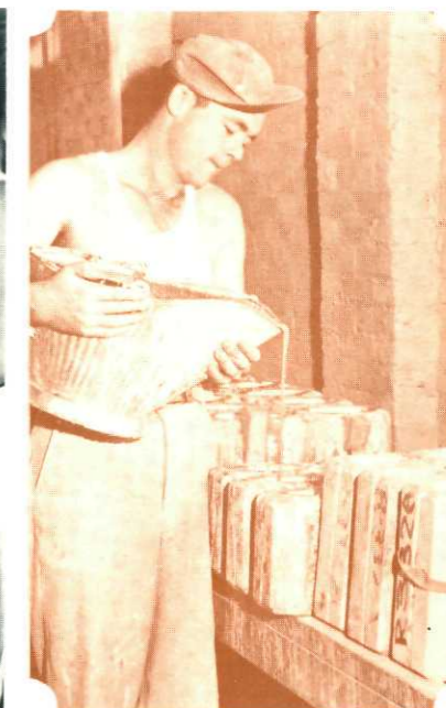
As a contrast, above is shown the early, slow process of carrying and pouring slip.
