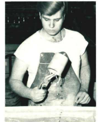
Highly developed glazes are applied by hand to each piece to assure fine quality.
