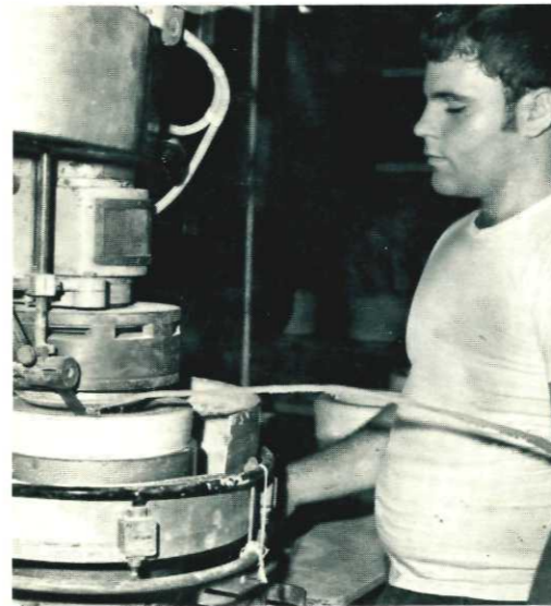
An automatic jigger wheel which produced automatically a piece of pottery according to the inside of the mold.
