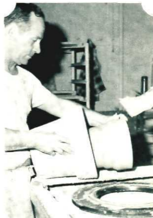
A jigger wheel is the outgrowth of a potter's wheel. Here we use a Plaster of Paris mold and a putty-like clay and form the piece of pottery according to the inside of the mold.
