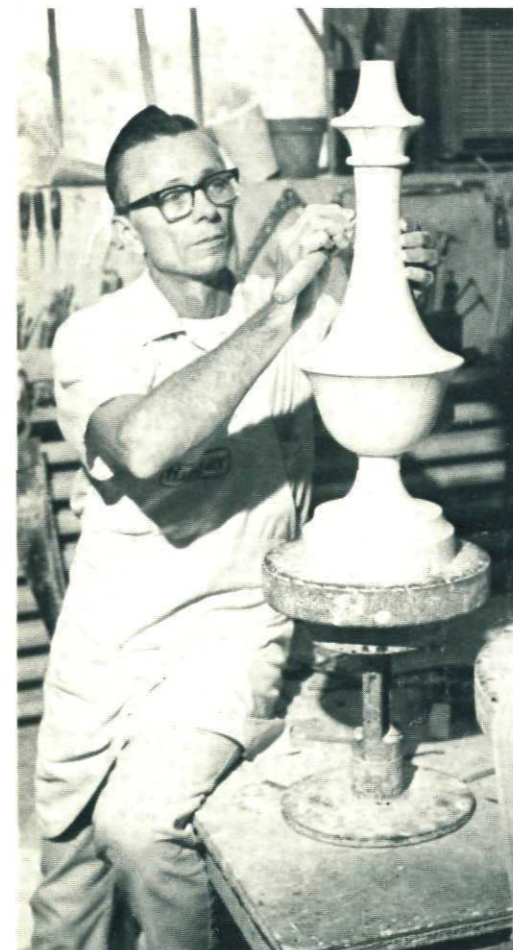
Precise models have to be made for those pieces that will eventually be produced.
