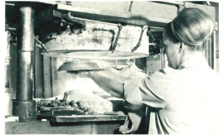
Certain hollow-ware designs can be made by a pressing process. Haeger uses this on certain items.
