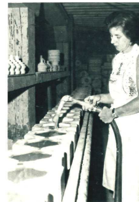
Slip, liquid clay, is pumped into production molds.
