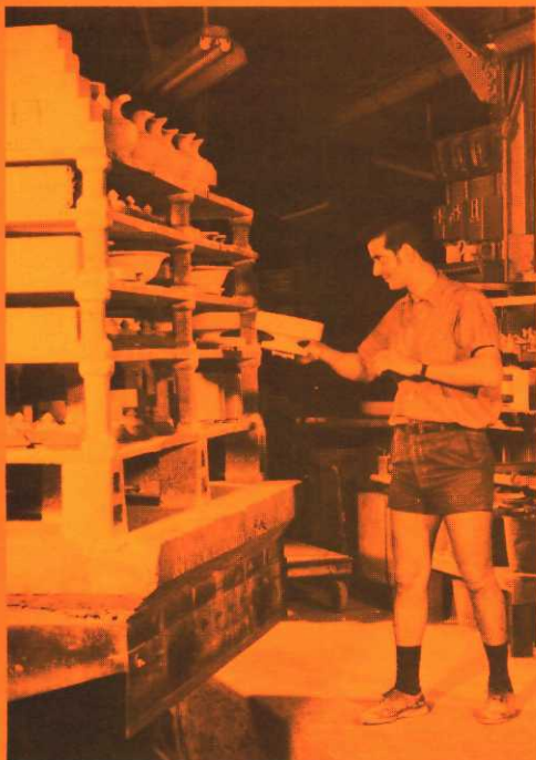
When the glaze has dried, kiln cars are loaded with ware to be fired.
