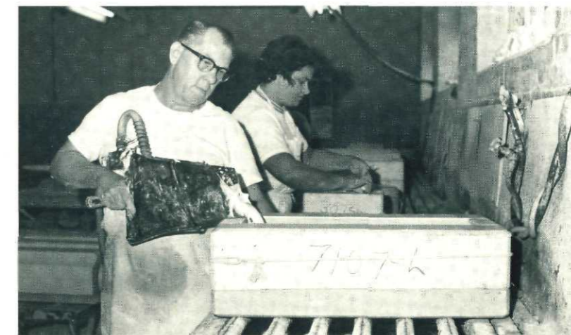
The block and case is being poured with plaster in order that production molds can be produced.
